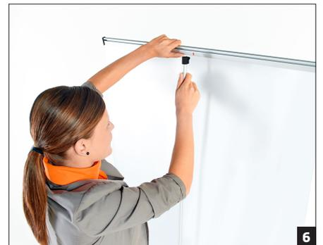
Using the hook, gently and carefully fix the clamping rail to the support bar.
