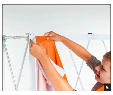
Attach the print to the Velcro tape. Start with one of the corners on the front of the system, pull the print tight and stretch it across to the adjacent corner. Continue in this way to fix the entire print to the front of the system.
